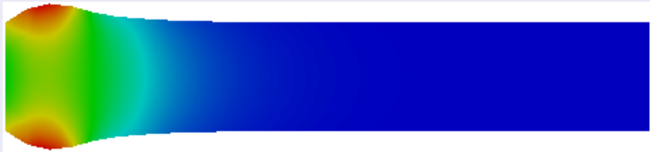
Figura: Pressure wave propagating through the blood vessel. The displacement is magnified five times.
