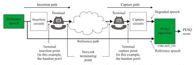
NOTE – Depending on how the signals are inserted, captured and stored, and whether the ITU-T Rec. P.862 measurement computations are done in real-time or deferred, these paths may be continuous physical electrical pathways, or they may be logical paths, such as when an output sample is stored for later analysis.
