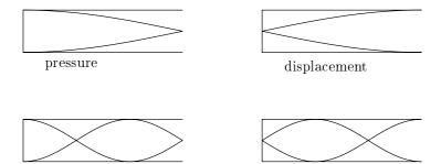
It follows that for closed tubes, odd multiples of the fundamental frequency dominate. For example, the flute is an open tube, so all multiples of the fundamental are present. The clarinet is a closed tube, so odd multiples predominate.
