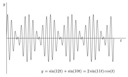
So for example, suppose that a piano tuner has tuned one of the three strings corresponding to the note A above middle C to 440 Hz. The second string is still out of tune, so that it resonates at 436 Hz. The third is being
