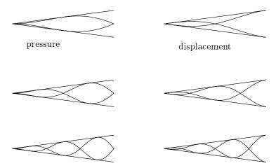
The oboe has a conical bore so again all multiples are present. This explains why the flute and oboe overblow at the octave, while the clarinet overblows at an octave plus a perfect fifth, which represents tripling the frequency. The odd multiples of the fundamental frequency dominate for a clarinet, although in practice there are small amplitudes present for the even ones from four times the fundamental upwards as well.
